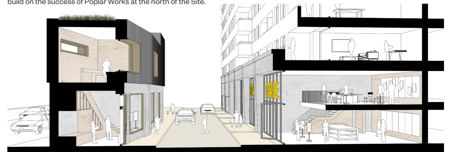
Fig.33 Section through Enterprise Yard showing the continuation of Poplar Works maker-spaces opposite a residential building with a plinth activating the ground floor and homes set back above
