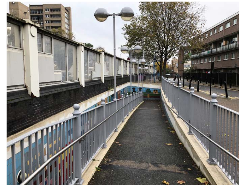
Fig.644 1:10 sloped access to the Pedestrian underpass
