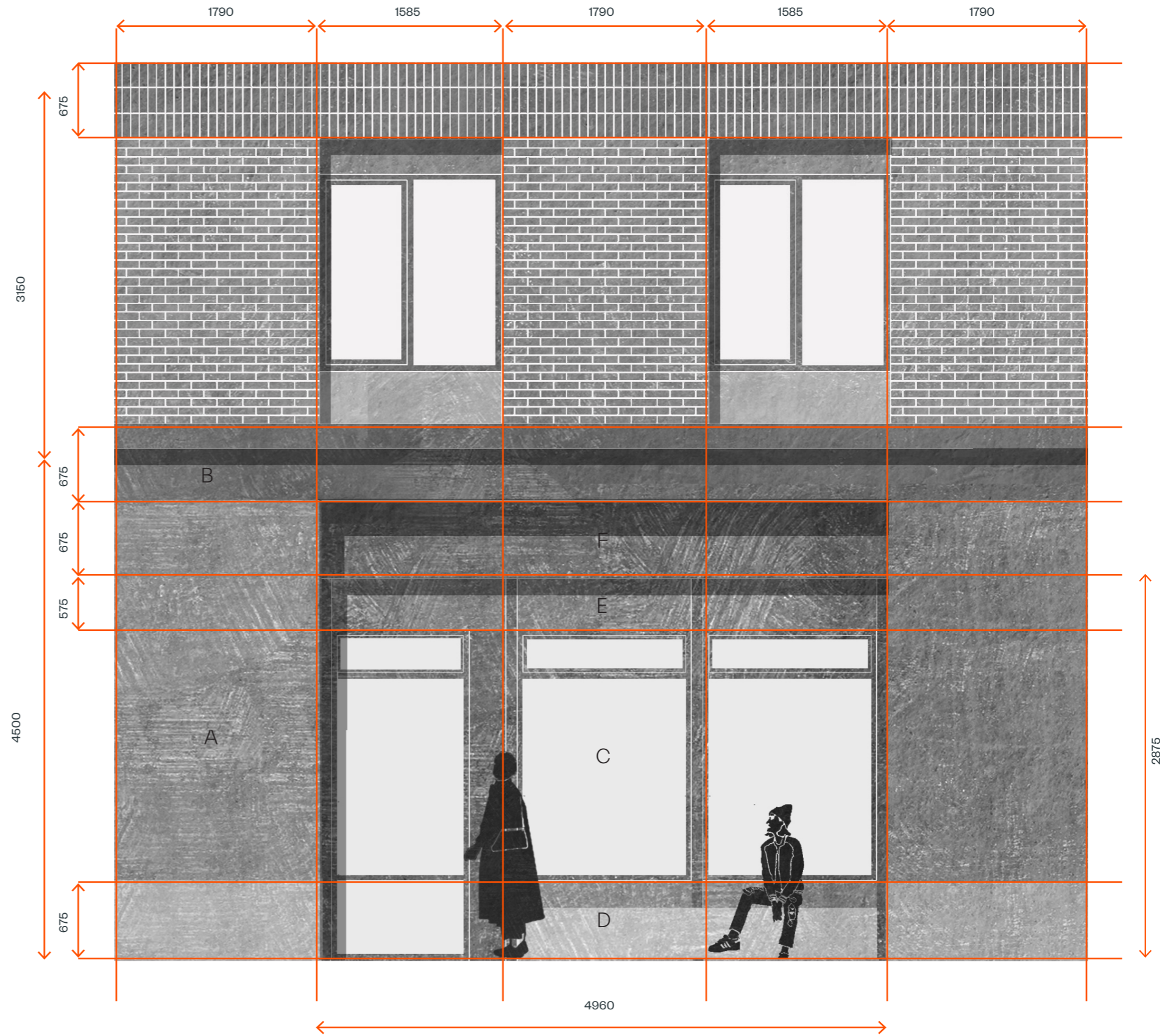
Coordinating datums of retail fronts and facade
