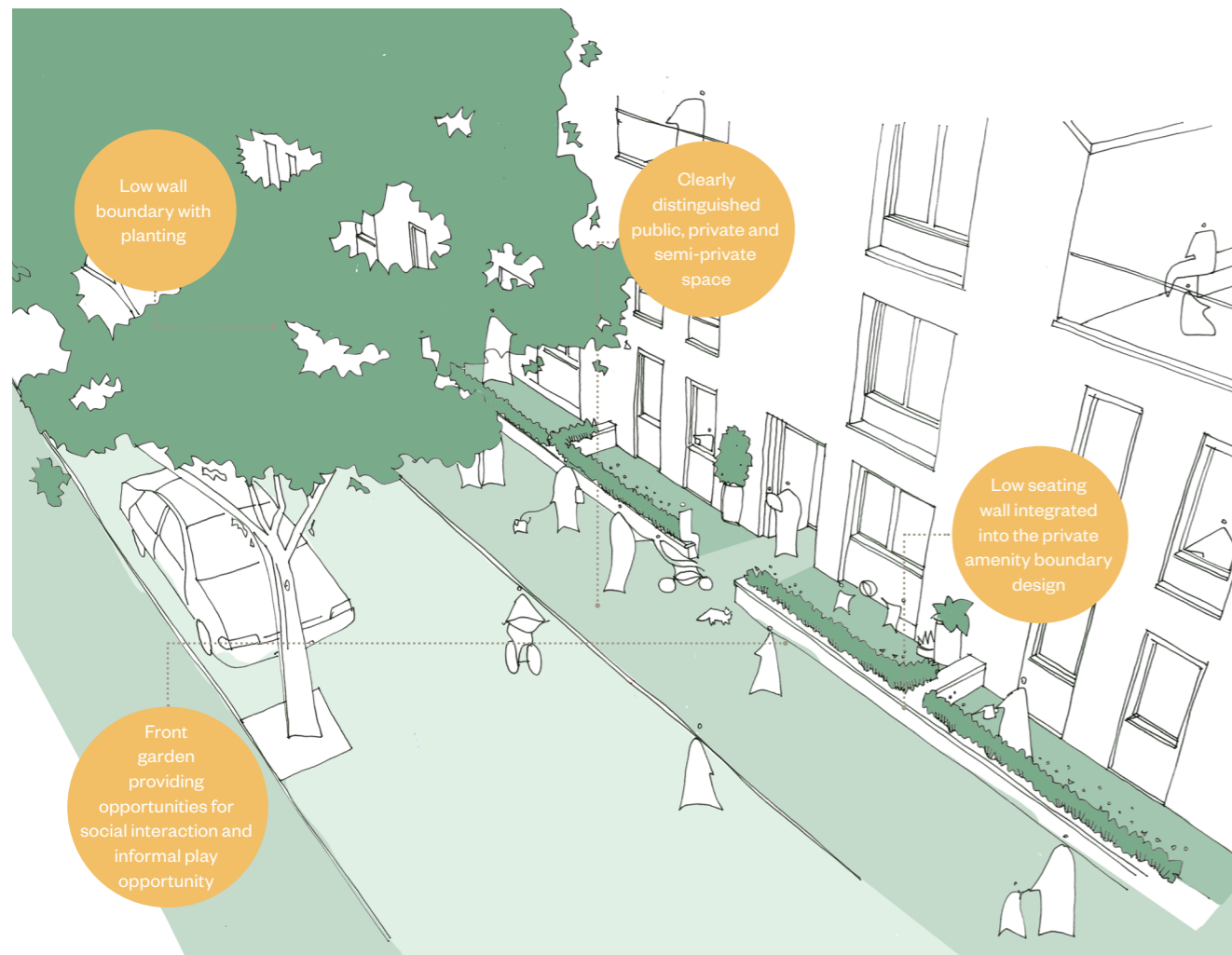
Fig.240 Residential thresholds along Community Lane
