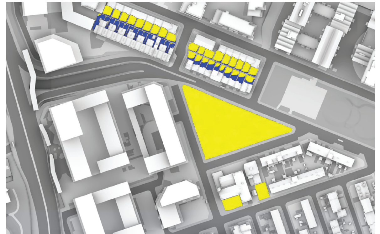
OVERSHADOWING ASSESSMENT - MAX PARAMETER - AREAS 1-46 SUN HOURS ON GROUND - BRE TEST
