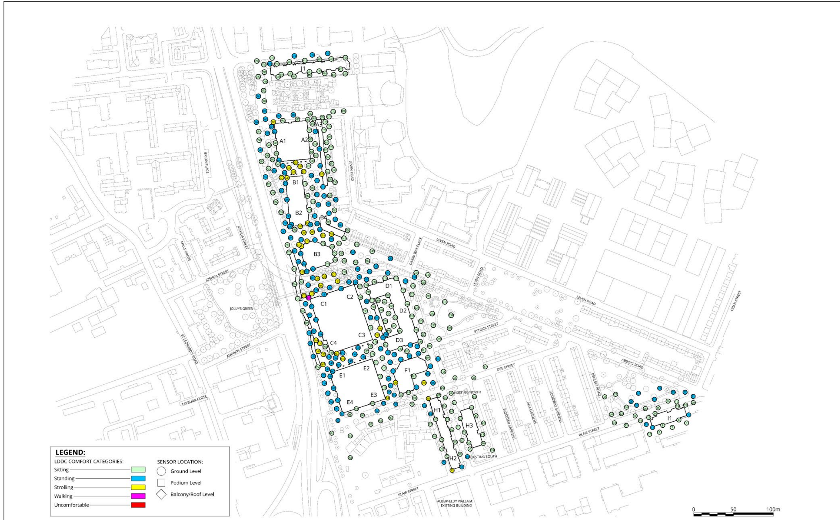
Figure 13.64 Configuration 10: Proposed Development (Illustrative Scheme) and Phase A with Cumulative Surrounding Buildings, Proposed Landscaping and Wind Mitigation Measures – Ground Level (Windiest Season)
