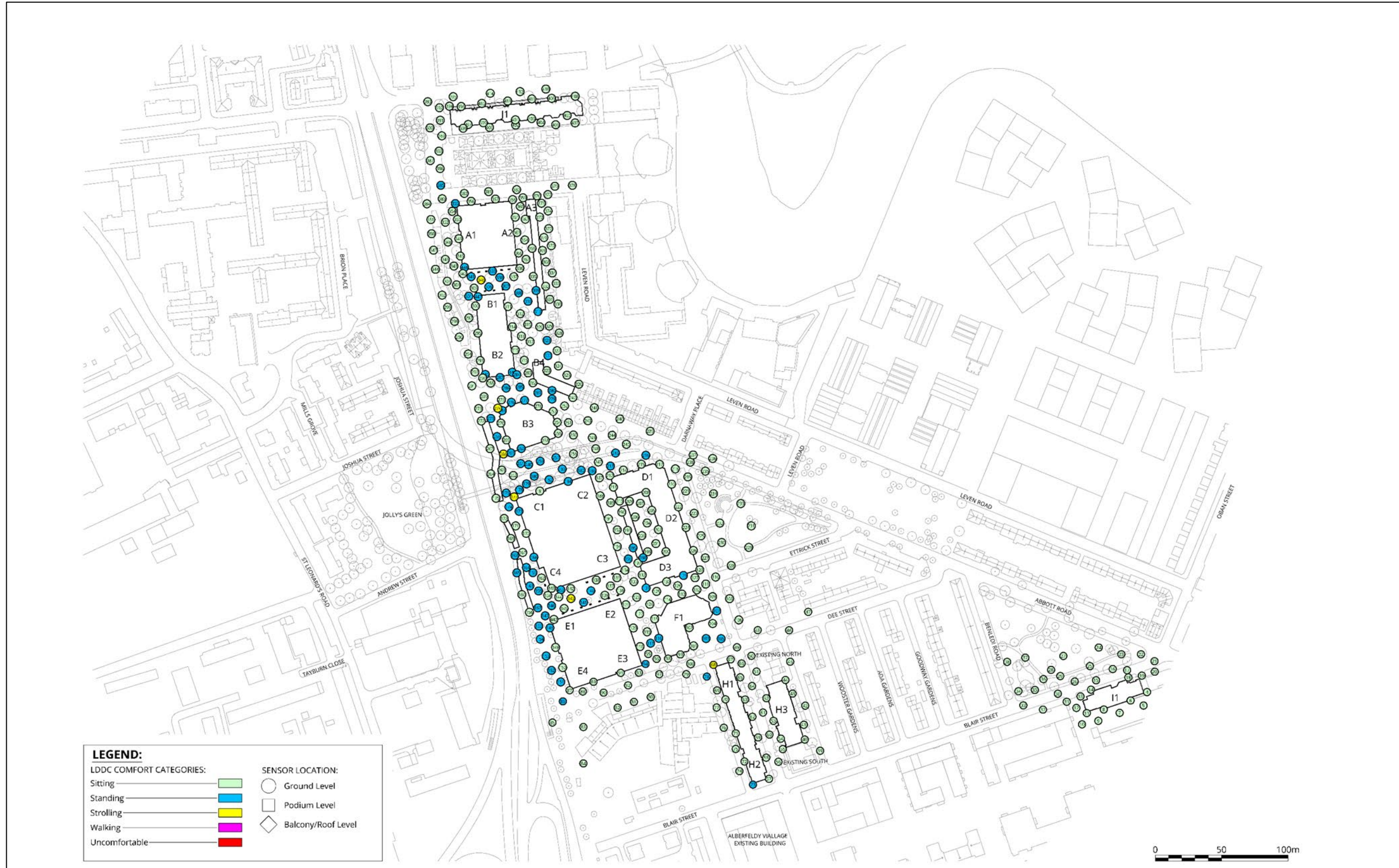
Figure 13.65 Configuration 10: Proposed Development (Illustrative Scheme) and Phase A with Cumulative Surrounding Buildings, Proposed Landscaping and Wind Mitigation Measures – Ground Level (Summer Season)
