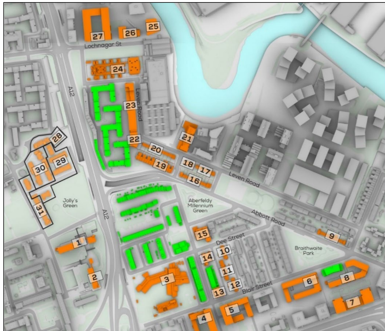
Figure 14.1 Existing Daylight and Sunlight Receptors
