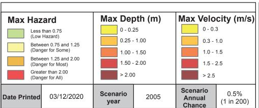
This map shows the level of flood hazard to people (called a hazard rating) if our flood defences are breached at certain locations, for a range of scenarios. The hazard rating depends on the depth and velocity of floodwater, and maximum values of these are also mapped.
