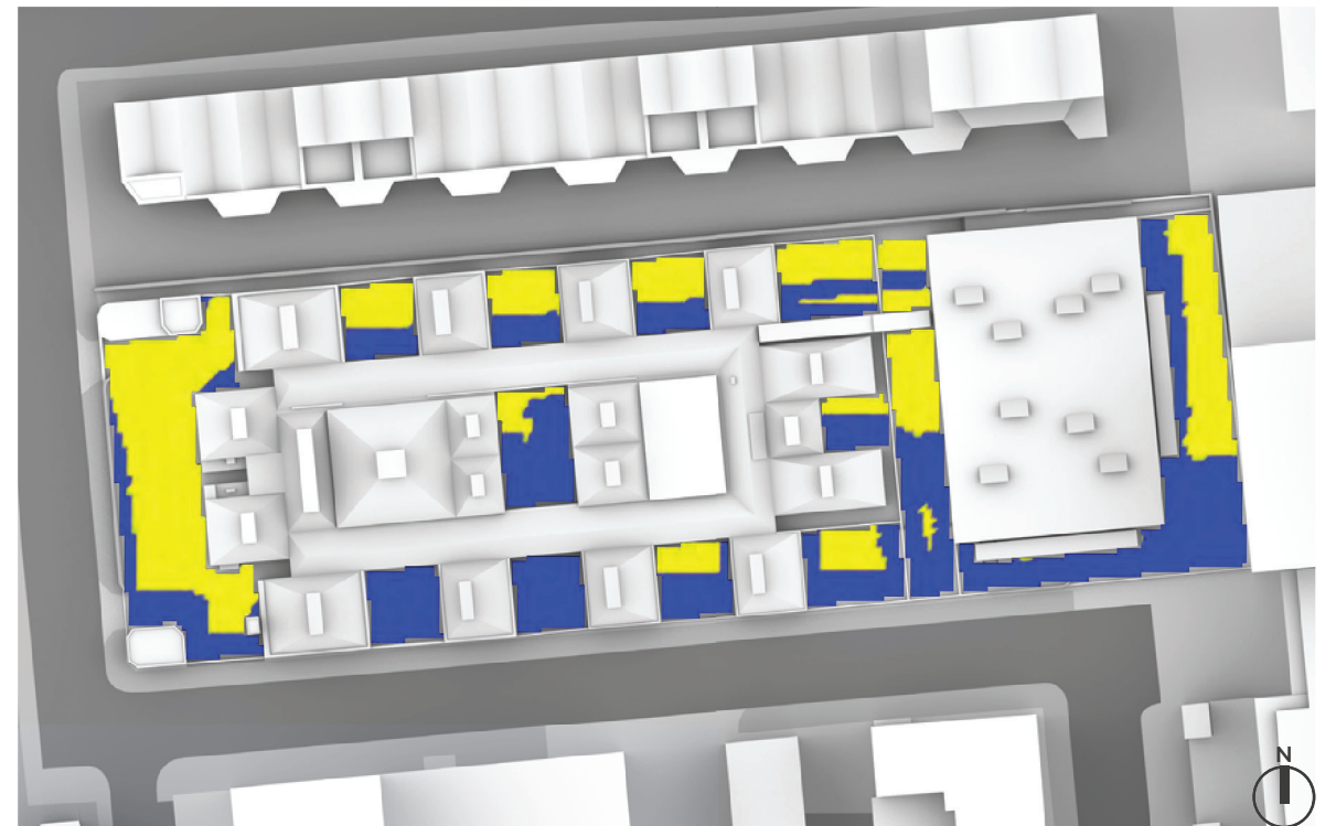
OVERSHADOWING ASSESSMENT - CUMULATIVE - AREAS 65-78 SUN HOURS ON GROUND - BRE TEST
