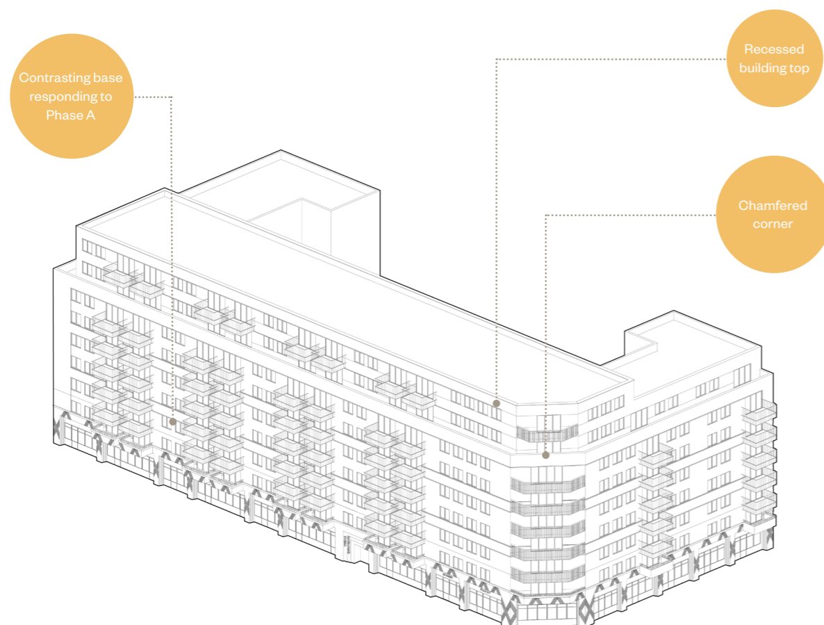
Fig.340 Isometric view of courtyard building addressing public space (Illustrative proposal)
