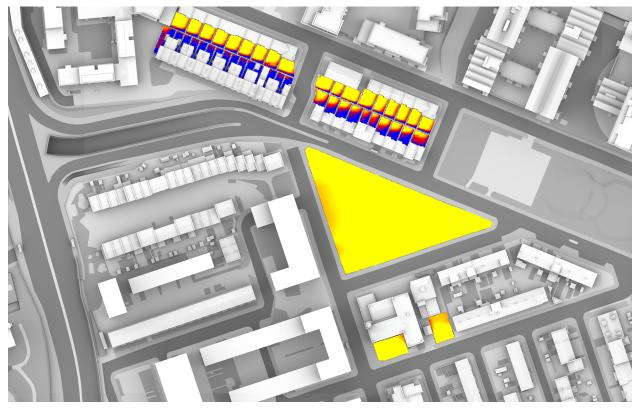
OVERSHADOWING ASSESSMENT - MAX PARAMETER - AREAS 1-46 SUN EXPOSURE ON GROUND - 21<sup>ST</sup> MARCH (SPRING EQUINOX)
