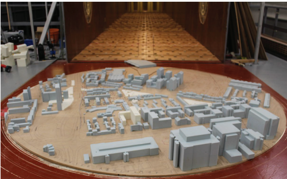
Figure 5: Existing Site with Existing Surrounding Buildings (Configuration 1, Board 2) – View in the Wind Tunnel (from the south)
