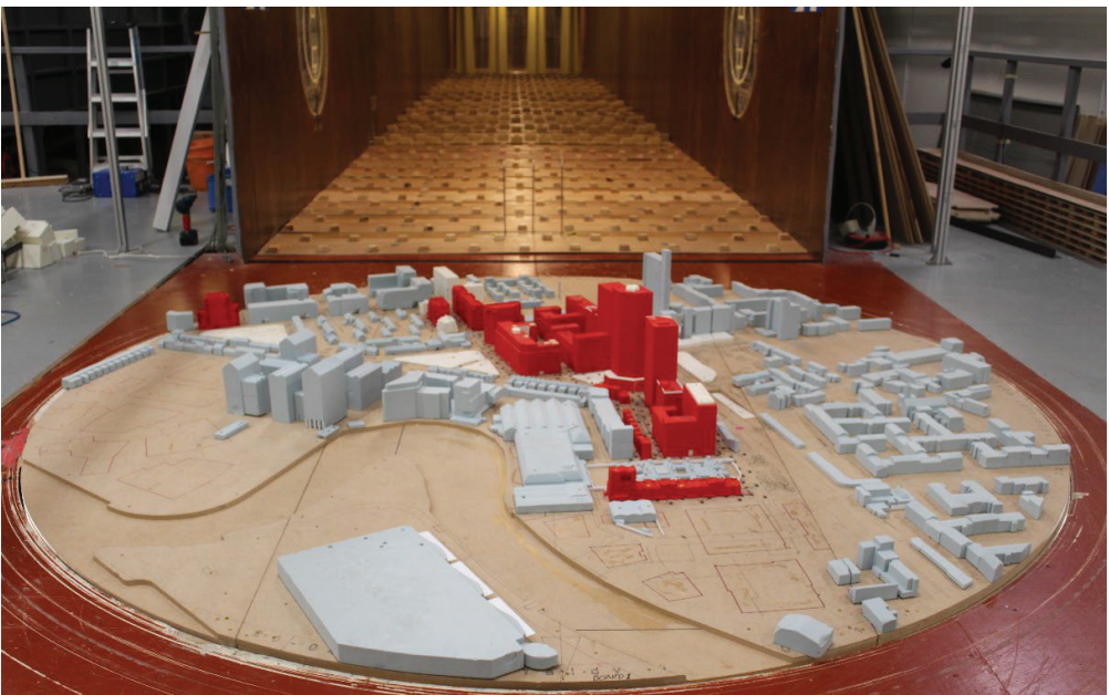
Figure 15: Proposed Development (Illustrative Scheme) and Phase A with Existing Surrounding Buildings (Configuration 4, Board 1) – View in the Wind Tunnel (from the north)
