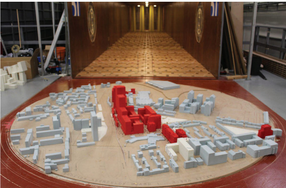
Figure 11: Proposed Development (Outline Proposals plus Detailed Proposals) with Existing Surrounding Buildings (Configuration 3, Board 1) – View in the Wind Tunnel (from the south)
