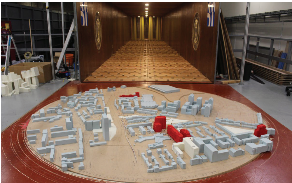
Figure 7: Detailed Proposals (Phase A) with Existing Surrounding Buildings (Configuration 2, Board 1) – View in the Wind Tunnel (from the south)
