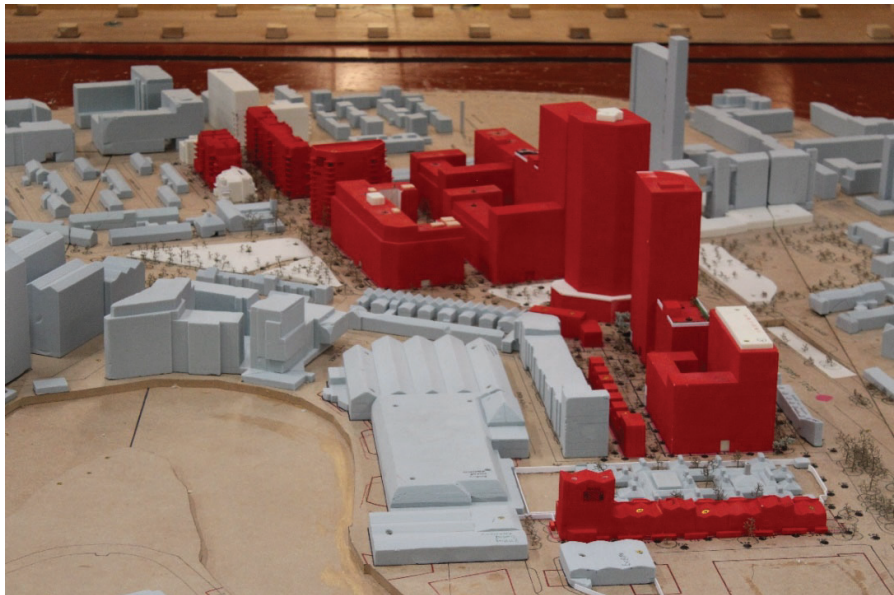
Figure 18: Proposed Development (Illustrative Scheme) and Phase A with Existing Surrounding Buildings, Proposed Landscaping and Wind Mitigation Measures (Configuration 5, Board 1) – View in the Wind Tunnel (from the north)
