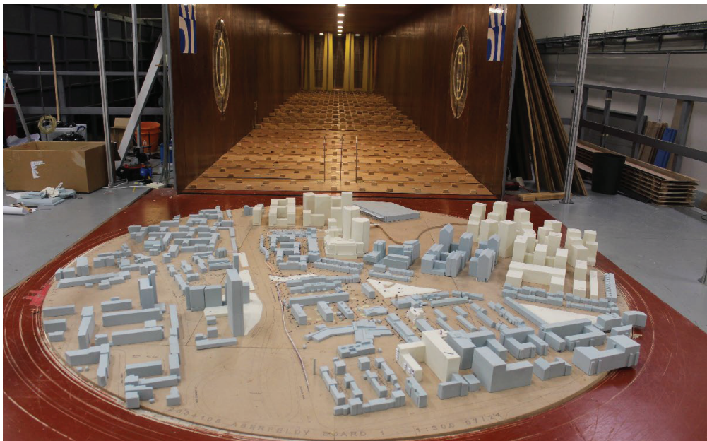
Figure 19: Existing Site with Cumulative Surrounding Buildings (Configuration 6, Board 1) – View in the Wind Tunnel (from the south)
