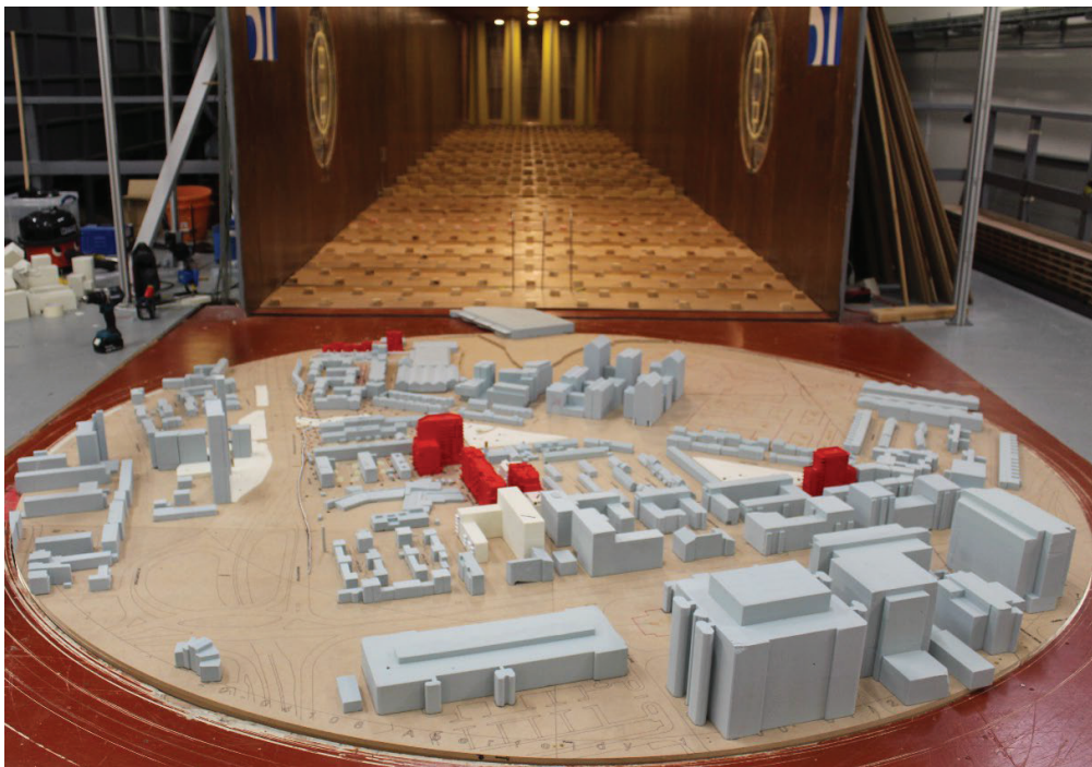
Figure 9: Detailed Proposals (Phase A) with Existing Surrounding Buildings (Configuration 2, Board 2) – View in the Wind Tunnel (from the south)
