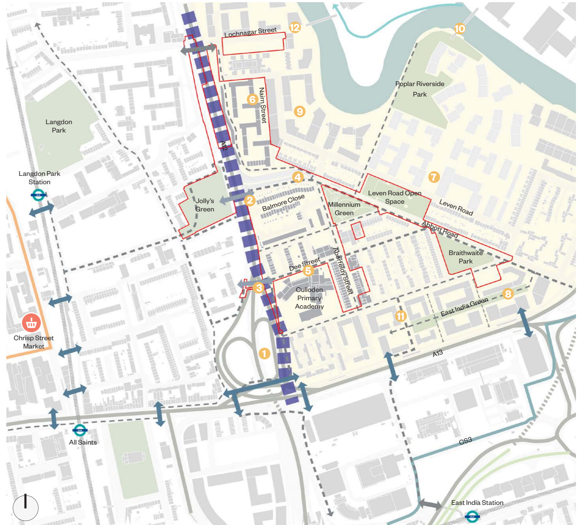
Fig.120 Plan showing existing pedestrian connections and the severance caused by the A12
