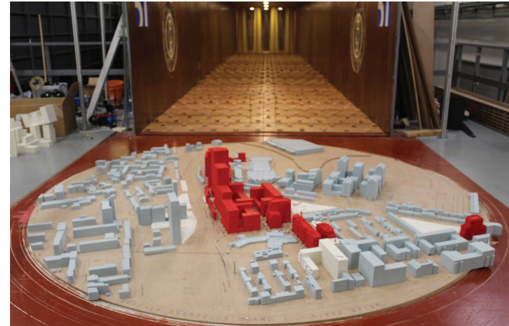
Figure 11: Proposed Development (Outline Proposals plus Detailed Proposals) with Existing Surrounding Buildings (Configuration 3, Board 1) – View in the Wind Tunnel (from the south)
