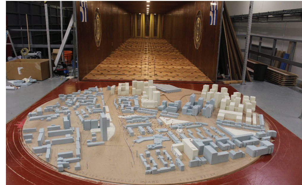
Figure 19: Existing Site with Cumulative Surrounding Buildings (Configuration 6, Board 1) – View in the Wind Tunnel (from the south)
