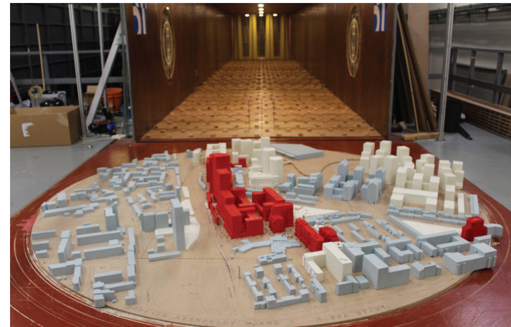
Figure 27: Proposed Development (Outline Proposals plus Detailed Proposals) with Cumulative Surrounding Buildings (Configuration 8, Board 1) – View in the Wind Tunnel (from the south)
