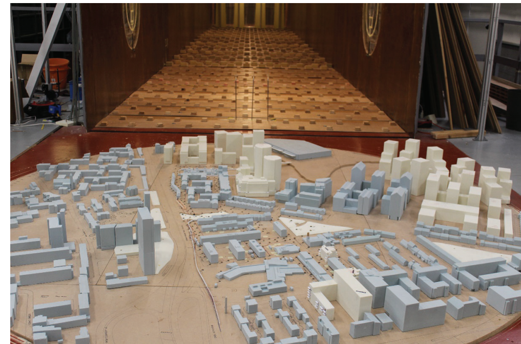
Figure 20: Existing Site with Cumulative Surrounding Buildings (Configuration 6, Board 1) – View in the Wind Tunnel (from the south)
