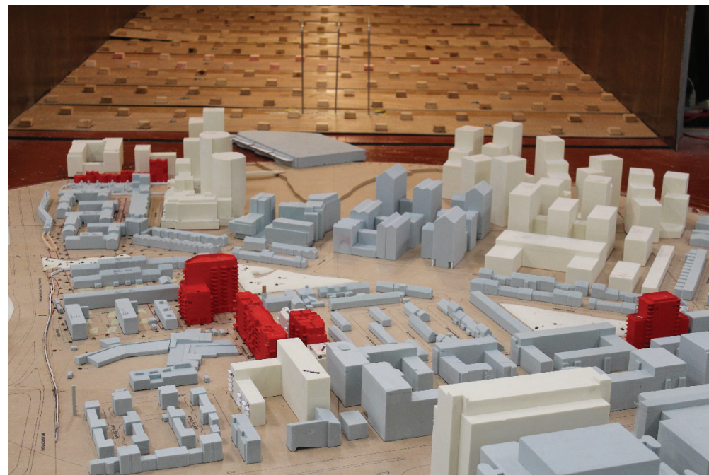
Figure 26: Detailed Proposals (Phase A) with Cumulative Surrounding Buildings (Configuration 7, Board 2) – View in the Wind Tunnel (from the south)
