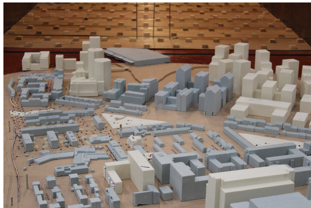
Figure 22: Existing Site with Cumulative Surrounding Buildings (Configuration 6, Board 2) – View in the Wind Tunnel (from the south)
