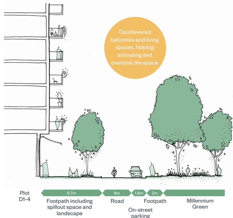
Fig.181 Illustrative section AA - Aberfeldy Street North
