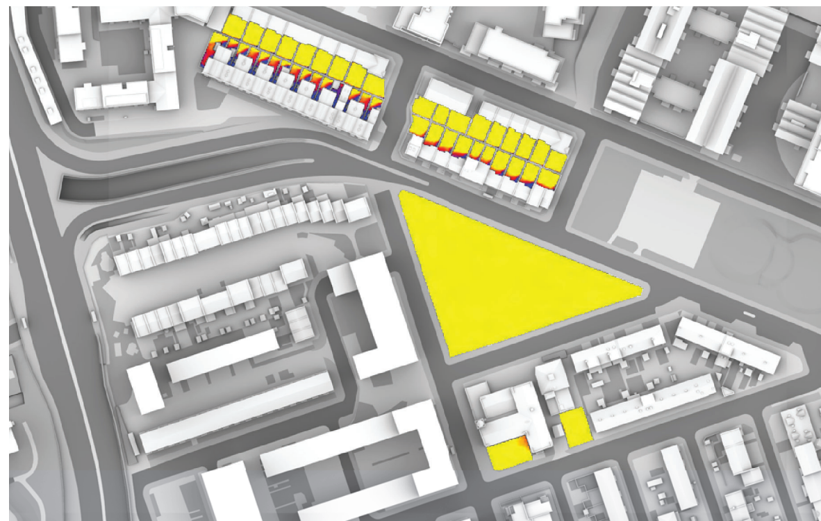
OVERSHADOWING ASSESSMENT - MAX PARAMETER - AREAS 1-46 SUN EXPOSURE ON GROUND - 21 ST JUNE (SUMMER SOLSTICE)
