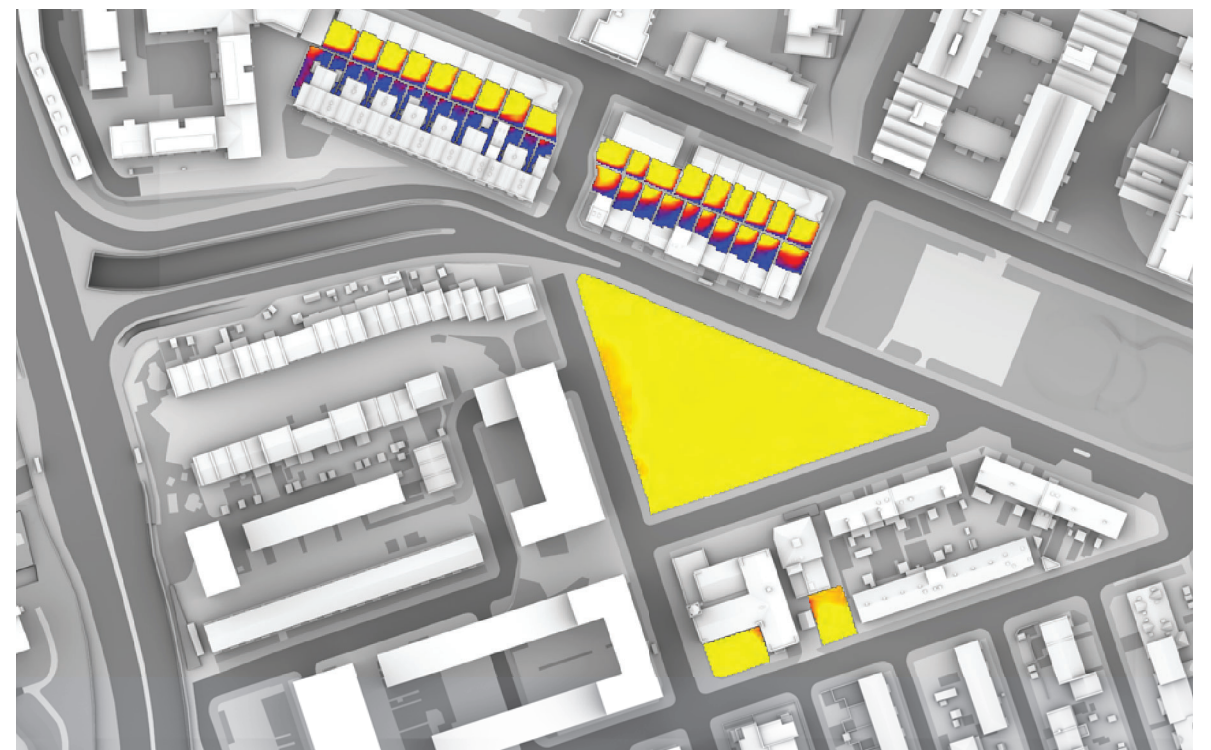
OVERSHADOWING ASSESSMENT - MAX PARAMETER - AREAS 1-46 SUN EXPOSURE ON GROUND - 21 ST MARCH (SPRING EQUINOX)
