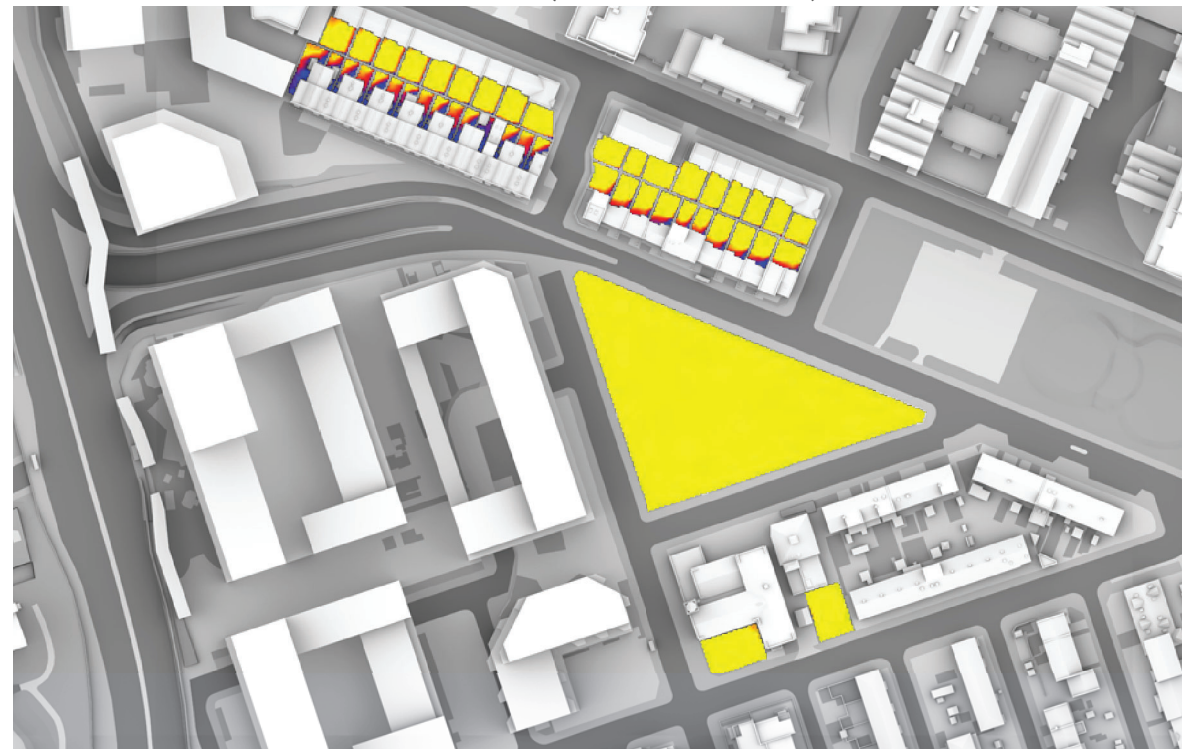
OVERSHADOWING ASSESSMENT - MAX PARAMETER - AREAS 1-46 SUN EXPOSURE ON GROUND - 21 ST JUNE (SUMMER SOLSTICE)
