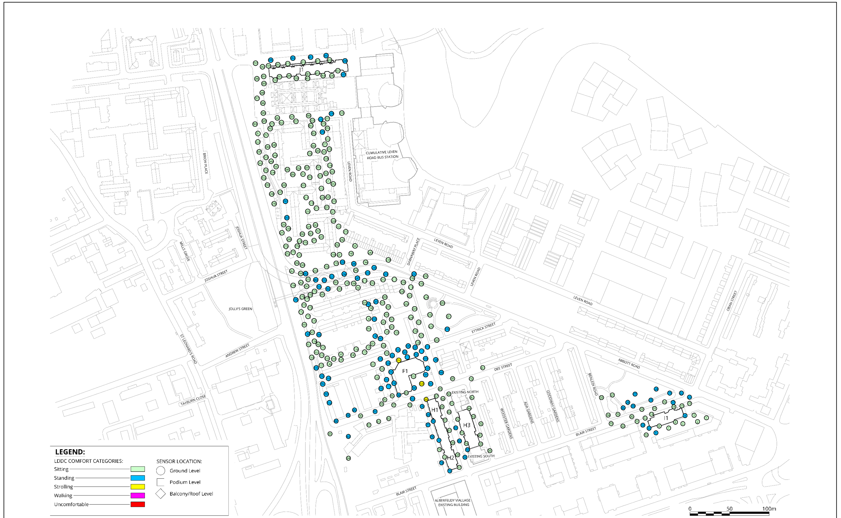
Figure 13.39 Configuration 7: Detailed Proposals (Phase A) with Cumulative Surrounding Buildings – Ground Level (Windiest Season)
