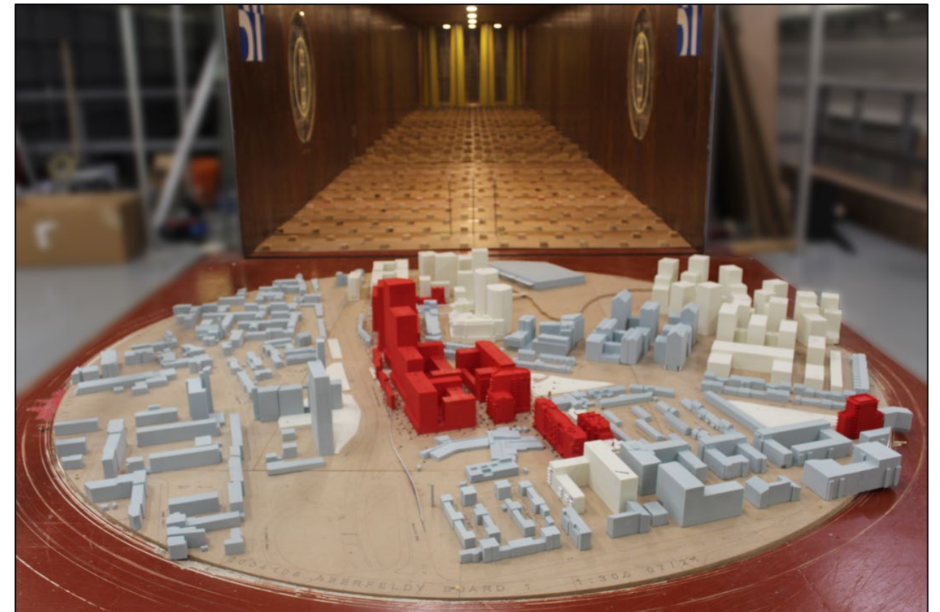
Figure 13.1 View from the south of the Proposed Development (Outline Proposals plus Detailed Proposals) with Cumulative Surrounding Buildings in the wind tunnel (Configuration 8)
