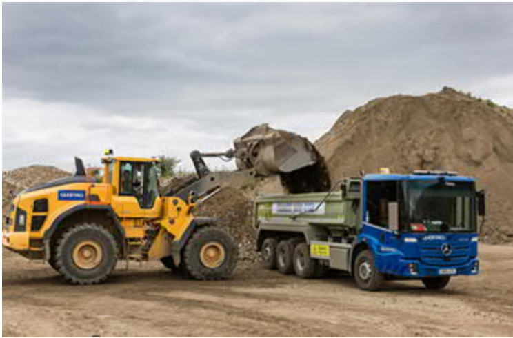
Figure 5-3 Example 32-Tonne Tipper Lorry
