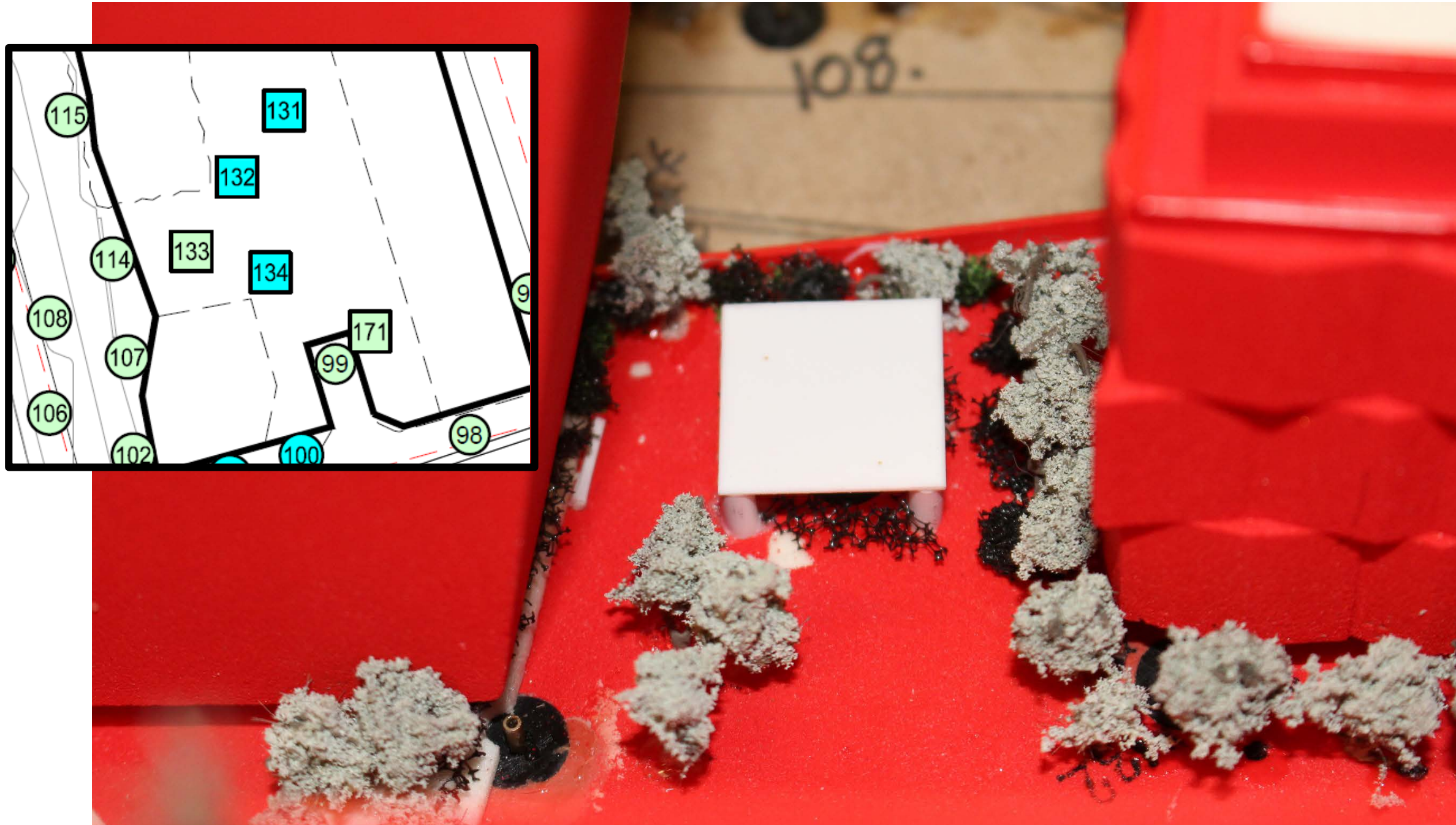
Figure 24: Example of a localized canopy of 2.5m height, with 1.5m shrubs around the perimeter, placed on probe 133.
