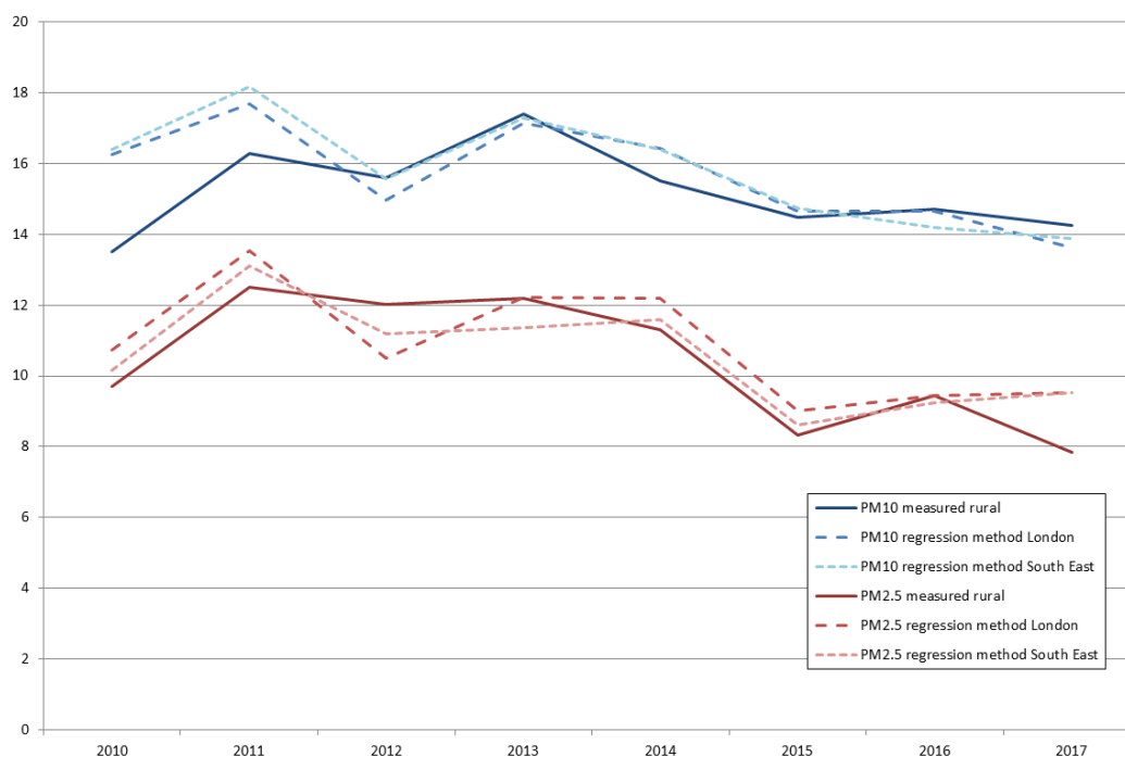
Figure 6: Time series of regional background PM 10 and PM 2.5 concentrations using three methods, after correcting for wood burning.
