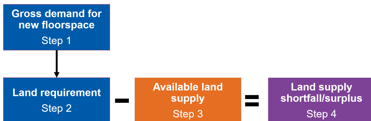
Figure 3-2: Summary of overarching approach used to quantify industrial floorspace and land demand
