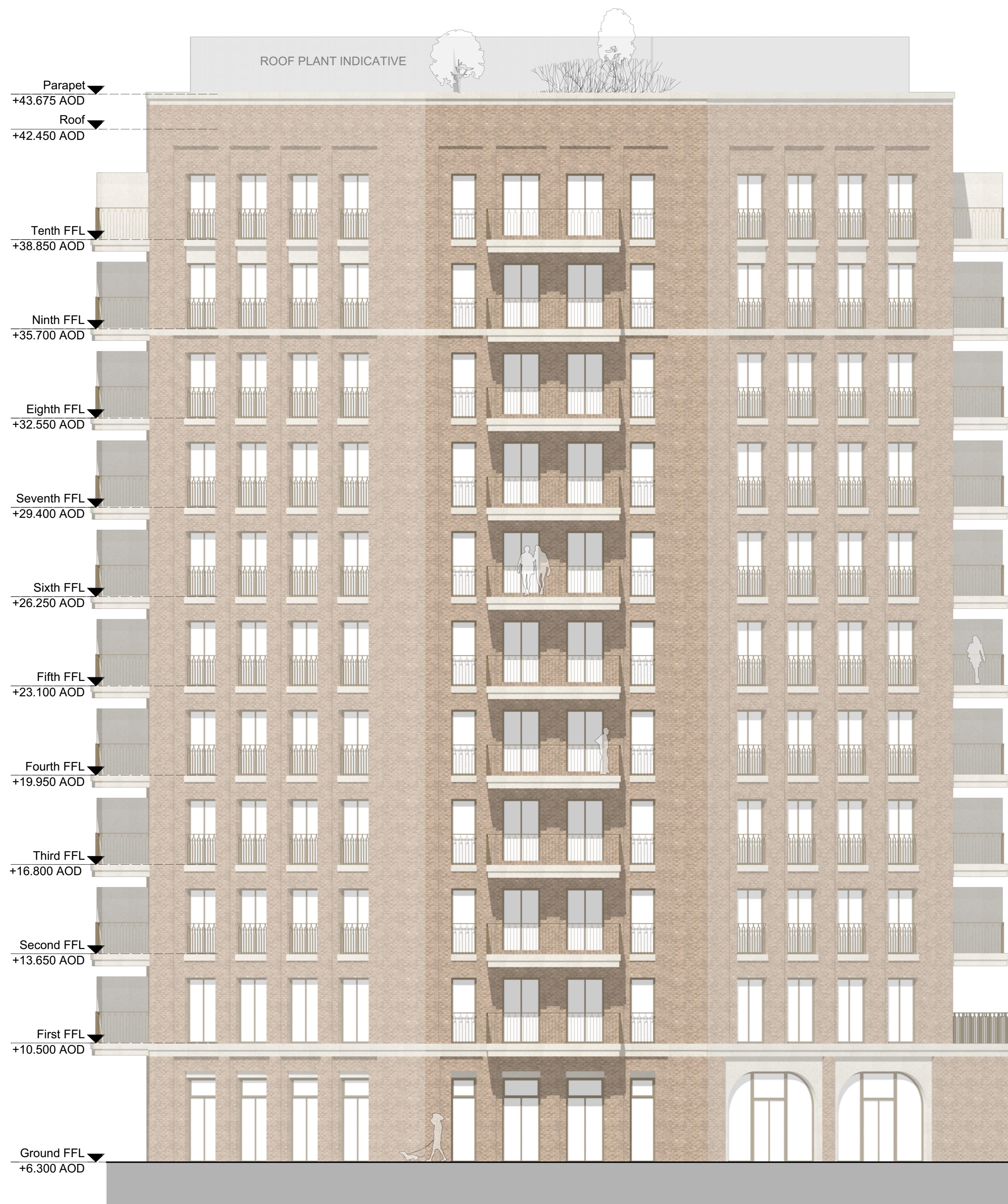
3 Block B South East Elevation Scale: 1:100
