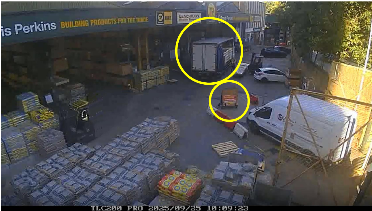
Figure 12 – HGV for inbound deliveries standing in yard / forklift offloading materials – with stop board deployed
