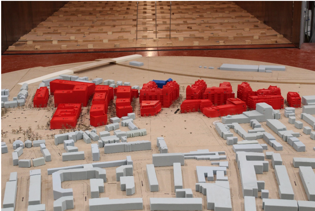
Figure 13 - Proposed Development with Landscaping and Existing Surrounding Buildings (Configuration 2) - View in the Wind Tunnel (from the South)
