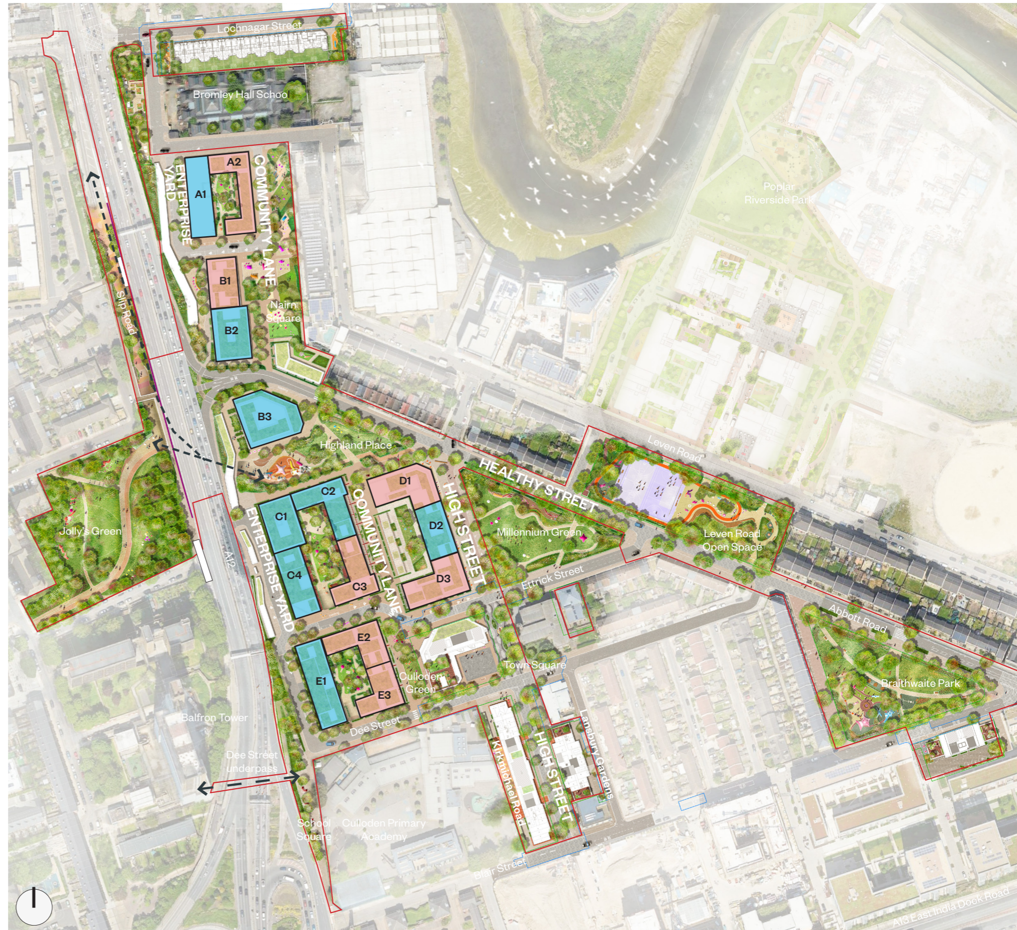
Fig.39 Plan showing the proposed layout of the illustrative masterplan and the buildings with the top floor of accommodation over 18m, and over 30m
