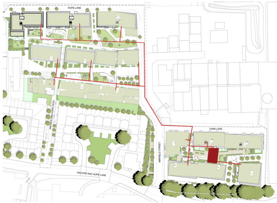
Figure 10: Indicative District Heat network routing
