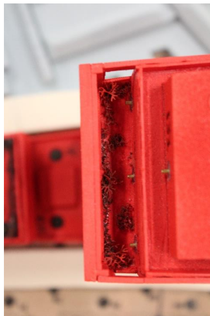
Figure 28: Proposed Development with Existing Surrounding Buildings and Wind Mitigation Measures (Configuration 3) – Wind Tunnel Photo
