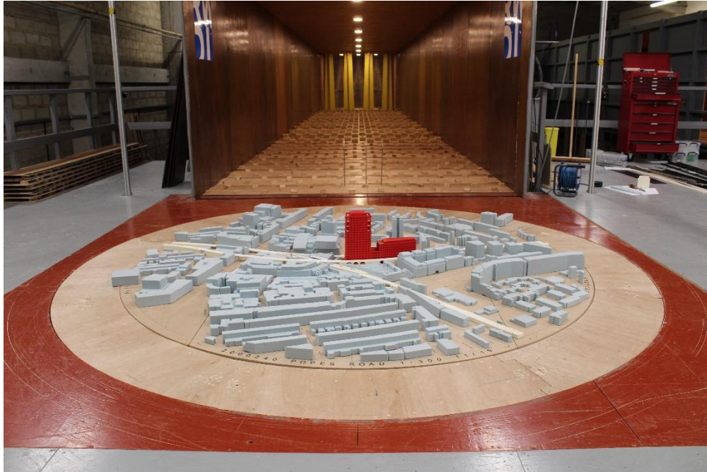
Figure 17: Proposed Development with Existing Surrounding Buildings (Configuration 2) - View in the Wind Tunnel (from the south)
