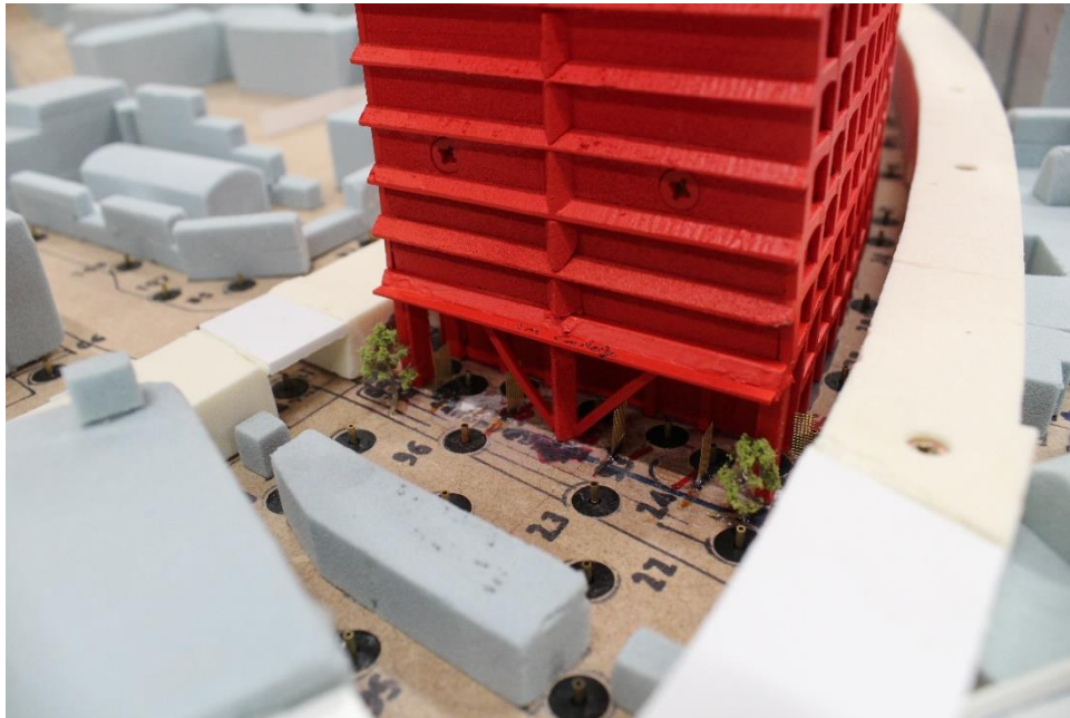
Figure 21: Proposed Development with Existing Surrounding Buildings and Wind Mitigation Measures (Configuration 3) - Wind Tunnel Photo
