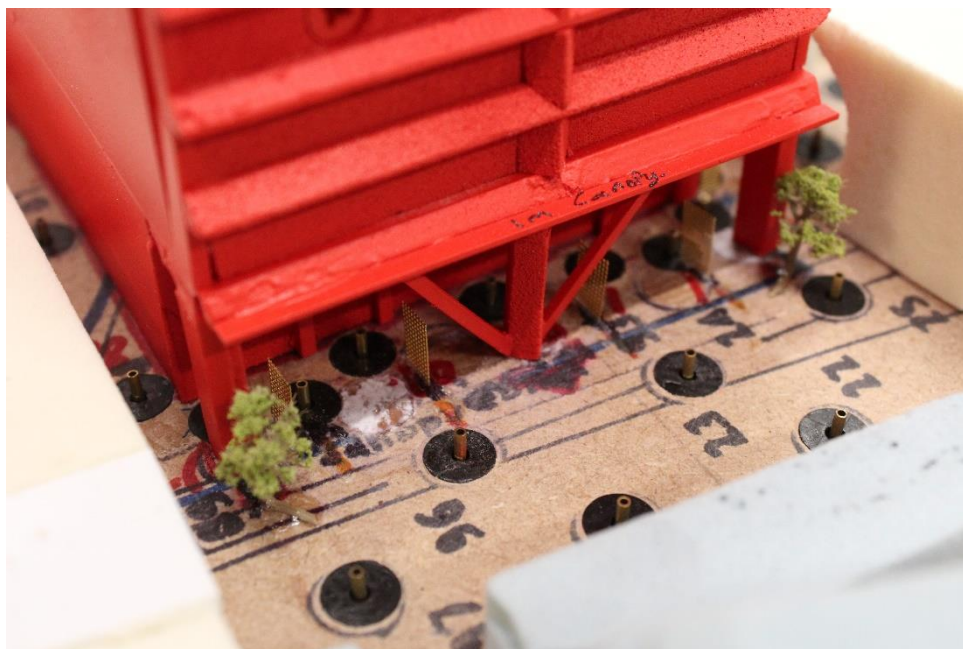
Figure 22: Proposed Development with Existing Surrounding Buildings and Wind Mitigation Measures (Configuration 3) - Wind Tunnel Photo
