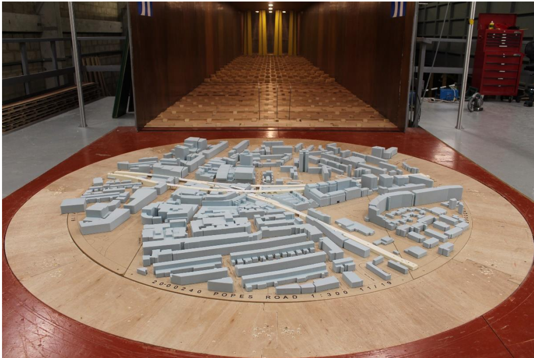
Figure 15: Existing Site with Existing Surrounding Buildings (Configuration 1) - View in the Wind Tunnel (from the south)
