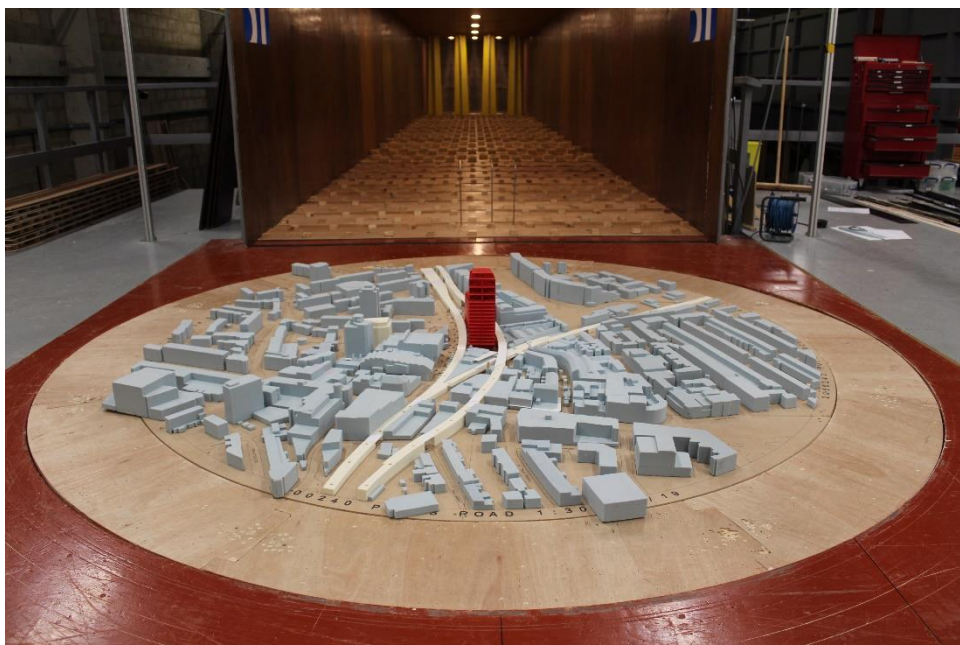
Figure 30: Proposed Development with Cumulative Surrounding Buildings and Wind Mitigation Measures (Configuration 4) - View in the Wind Tunnel (from the west)
