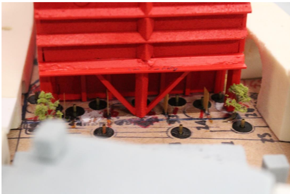
Figure 26: Proposed Development with Existing Surrounding Buildings and Wind Mitigation Measures (Configuration 3) - Wind Tunnel Photo
