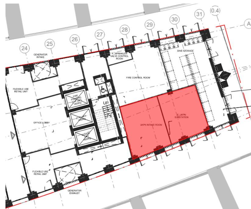
Figure 21 UKPN substation and intake room at ground floor level
