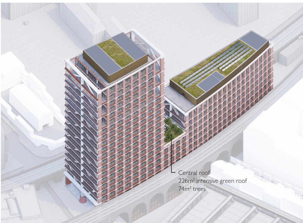
2.2 Axo diagram of proposal with additional intensive green roofs to east and west blocks
