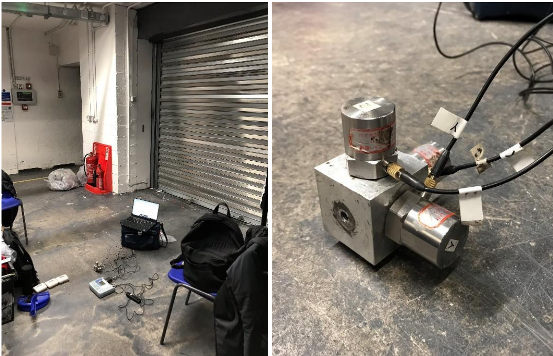
Figure 4 Vibration measurement location and equipment setup
