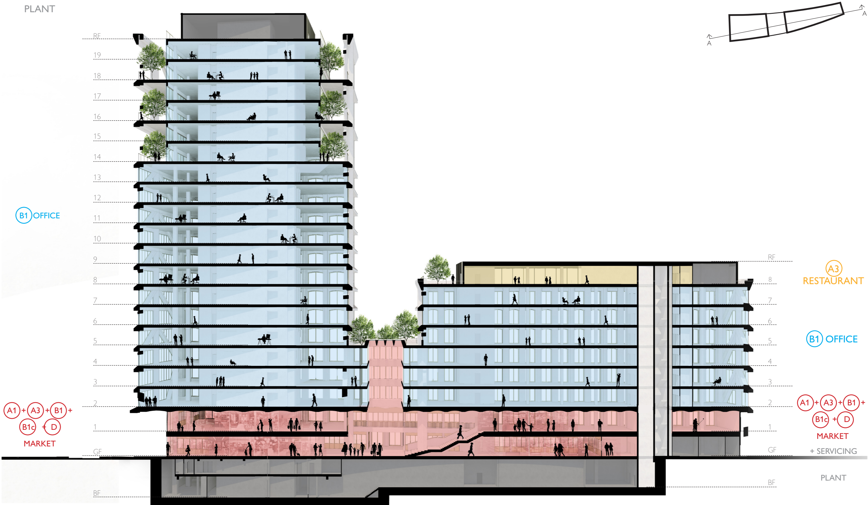
Fig. 2.3.1 Perspective Section Diagram of Building Uses
