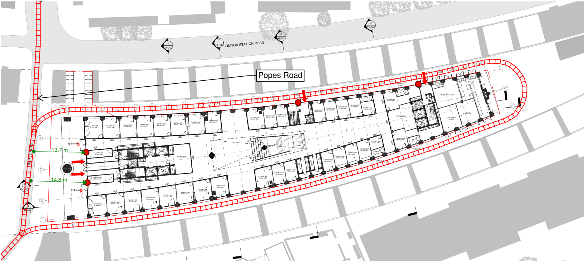
Figure 4: Indicative Fire Service Access Routes
