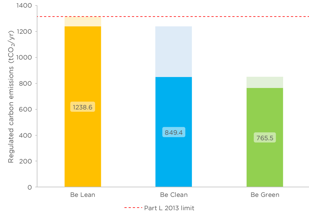
Figure 4.3 - Regulated CO 2 emissions after each stage of the energy hierarchy for the whole site
