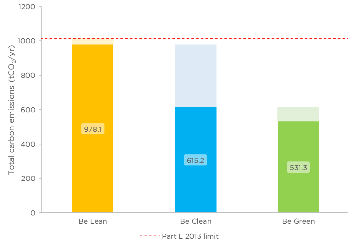
Figure 1.1 - Regulated CO 2 emissions after each stage of the energy hierarchy for domestic buildings
