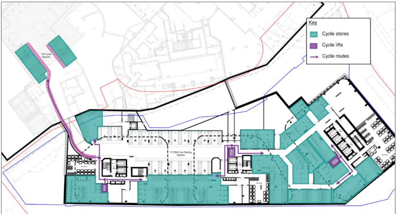
Figure 14: B1 long stay cycle parking layout and access
